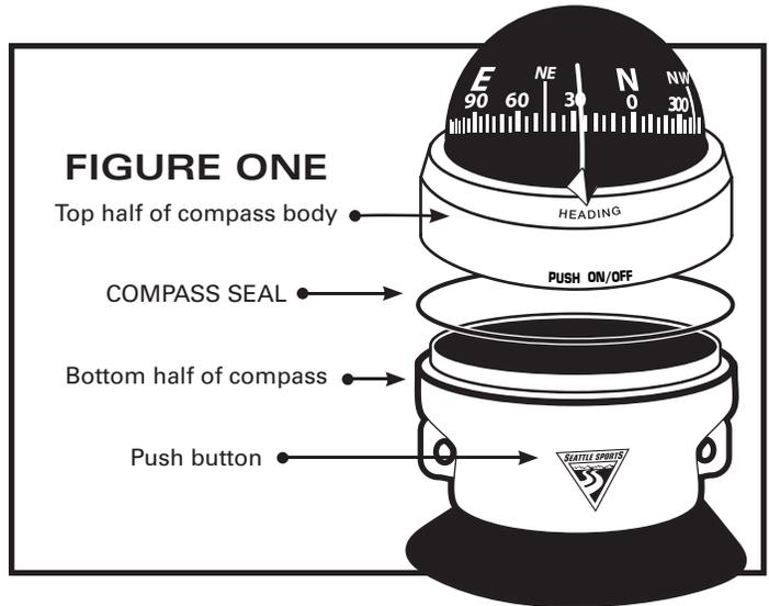
**NOTE:** The Seattle Sports triangle On/Off switch also lights up for added visibility and ease of turning on and off.
