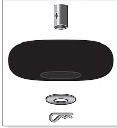
Foam pads are provided for hull protection. Put them on crossbars as shown below. Use soapy water or ArmorAll (do not use oil) on inside of foam to help it slide easily.
