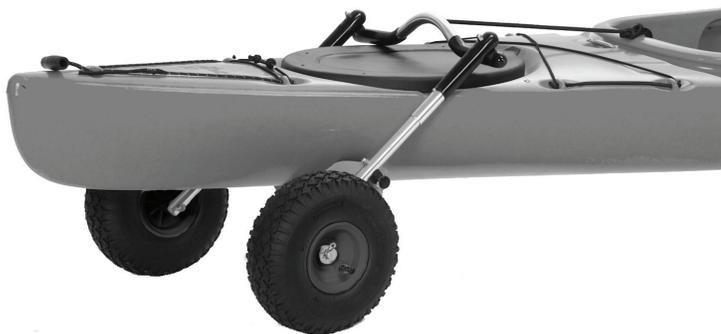
Unfold Original Air and attach wheels as illustrated. Place at one end of the craft. Use snap buttons to adjust the support arms to the second “click stop” from the top. Some of the snap button settings are behind the protective end caps. They can be located under the soft vinyl cap by pushing the button in and pulling up the support arm. Repeat on other arm.
